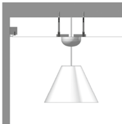
Sketch S39 - integration of lamp – distance > 10 mm
