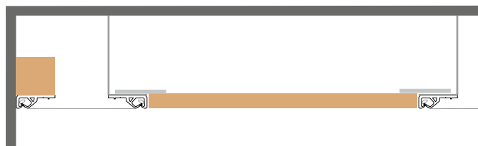
Sketch S36 - inspection cover - completed final assembly
