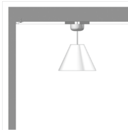
Sketch S38 - integration of lamp – distance = 10 mm
