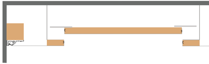
Sketch S33 - inspection cover without AP profile
